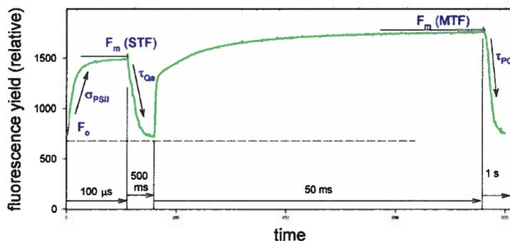
**Fluorescence Induction and Relaxation profile measured with the FIRE System**
